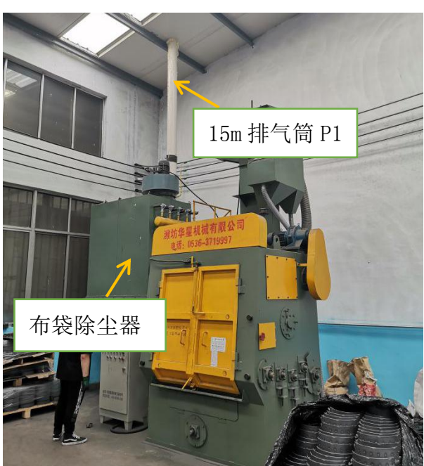
抛丸机+布袋除尘器+15m 排气筒 P1
